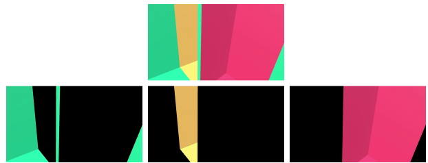
Figure 10: The user is standing in a green room looking at two portals to a yellow and a magenta room. The amount of rendering can in this case be divided by three if the pairs of cameras only render a masked out area of their room instead of the whole picture.
