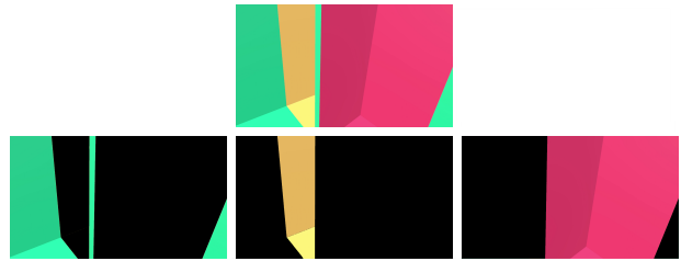
Figure 4: The user is standing in a green room looking at two portals to a yellow and a magenta room. The amount of rendering can in this case be divided by three if the pairs of cameras only render a masked out area of their room instead of the whole picture.
